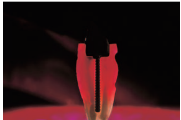
Figure 5.22 Sectioned incisor with a cast metal post and core showing that the latter impedes light transmission to the surrounding root.
